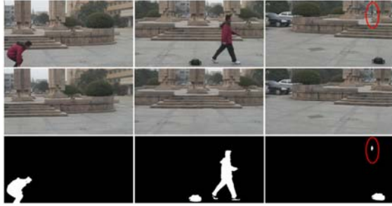
Figure 4: Results of the rotatable surveillance camera experiment. Top row: original video frames. Middle row: constructed backgrounds. Bottom row: extracted silhouettes.
