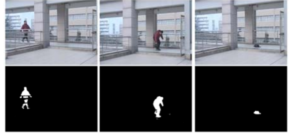
Figure 6: Results of the camera shaking experiment. Top row: original video frames. Bottom row: extracted silhouettes.
