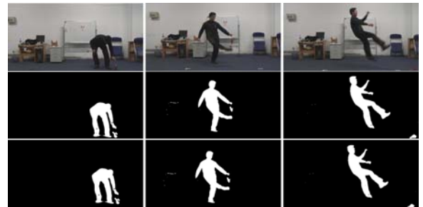
Figure 8: Results of stabilized silhouette generation. Top row: original video frames. Middle row: silhouettes before stabilizing. Bottom row: stabilized silhouettes.
